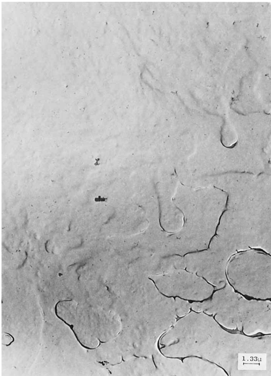
Fig. 12. Transmission electron micrograph of replica of PBT fracture surface. The smooth region of cohesive failure is visible at the upper left and the beginnings of patch fracture on the lower right.
