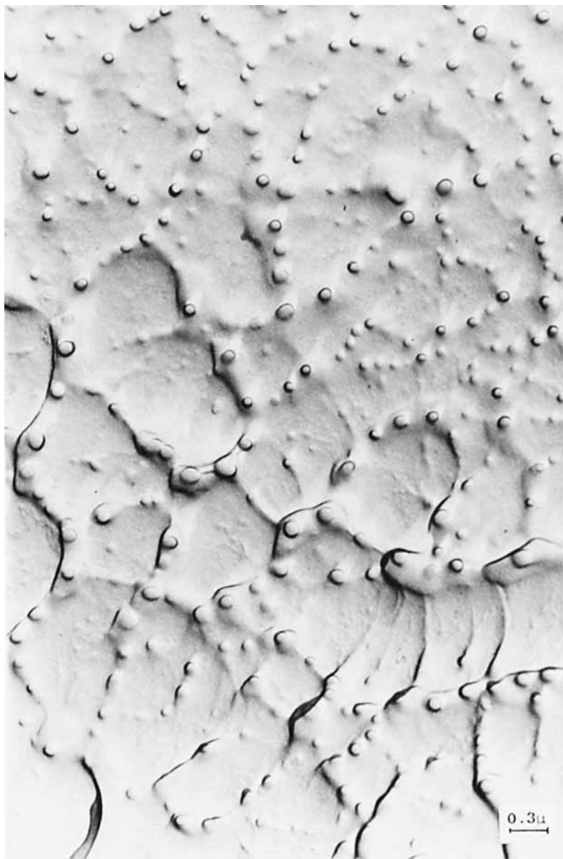
Fig. 14. Transmission electron micrograph of replica of PBT fracture surface. An enlargement of the nodular area in Figure 12 is shown.
