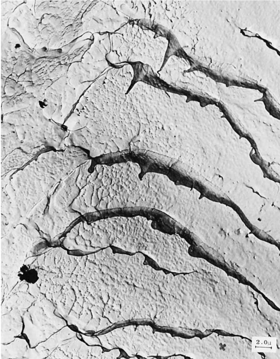
Fig. 13. Transmission electron micrograph of replica of PBT fracture surface. This area is \sim 200 \mu from the mirror zone and shows a characteristic mackerel fracture pattern and numerous small nodules of residual craze material.
